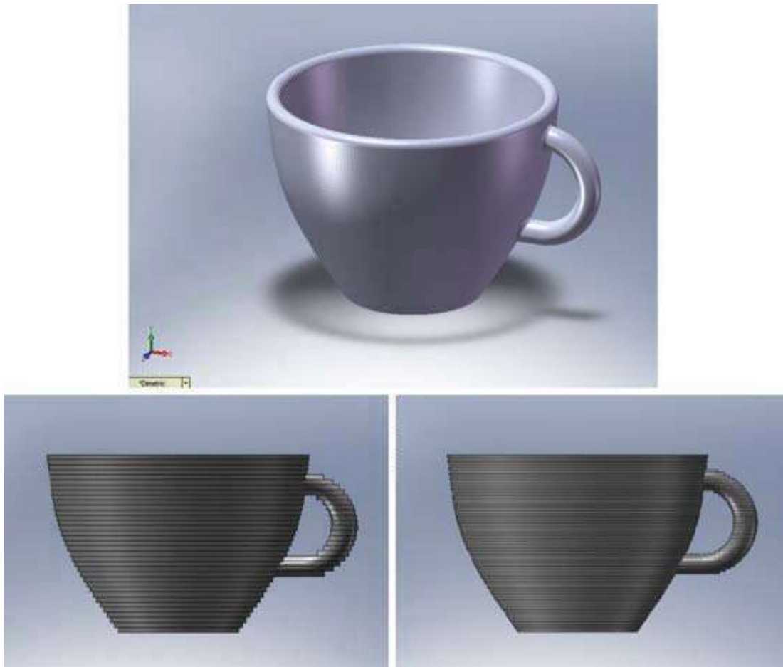
Fig. 1 CAD image of a teacup with further images showing the effects of building using different layer thicknesses
