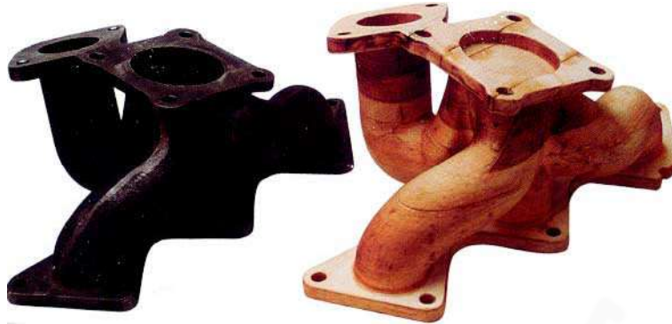
Figure 7.6: Cast metal (left) and RP pattern for sand casting (Courtesy of Helysis Inc.)
