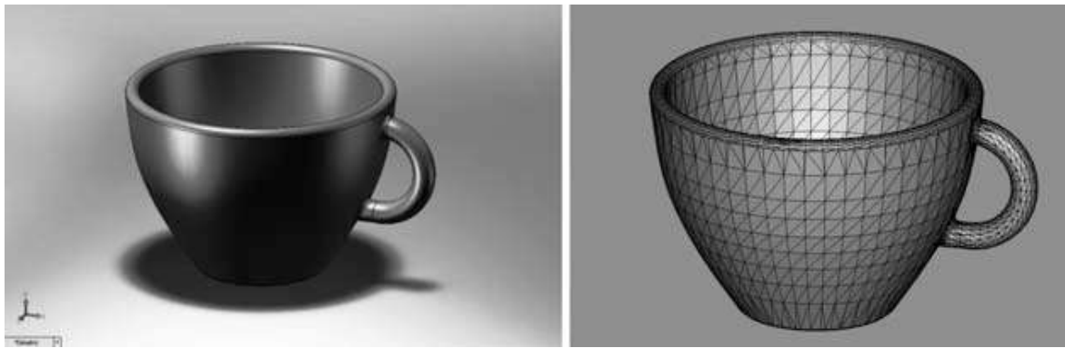
Fig. 5 A CAD model on the left converted into STL format on the right
